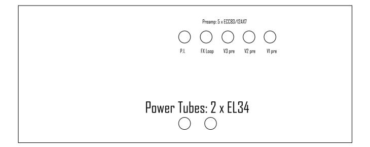
The life expectancy of the two EL34 power tubes depends on the average volume the amp works at, and can range from about 6 to 24 months. It is crucially important to replace them all at the same time, with high quality brand tubes. You will most likely need to adjust the bias with the internal trimmer.
