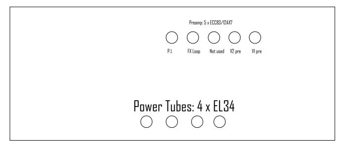
The life expectancy of the four E34L power tubes depends on the average volume the amp works at, and can range from about 12 to 48 months. It is crucially important to replace them all at the same time, with high quality brand tubes. You will most likely need to adjust the bias with the internal trimmer. Any short-circuits caused by a faulty tube can lead to burning one or more fuses, which must be replaced by **qualified MGD personnel and/or authorized technicians.**
